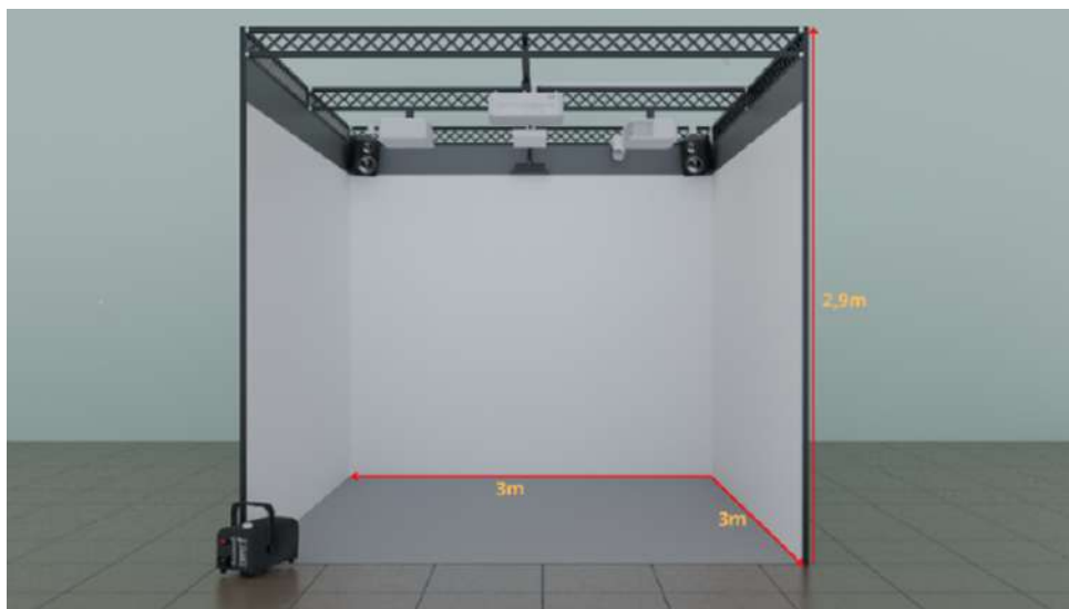
Figure 2 Front view of the 3×3-meter immersive booth design, illustrating projection walls, actuator placement, and user position
