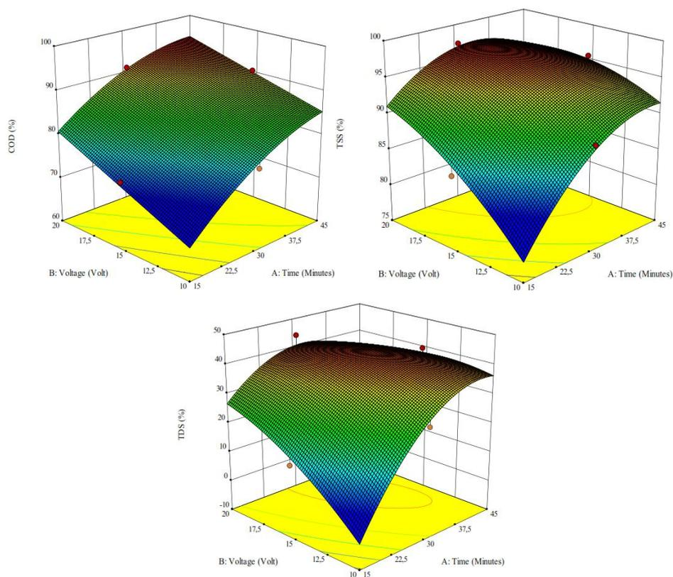
Figure 3 The effects of the voltage and time on COD, TSS, and TDS reduction without an electrolyte. Water reduction tended to occur more in the cathode compared to  $\text{Na}^+$ . Particles did not collide anymore, stopped growing, were not coagulated, and became stable. The  $\text{Cl}^-$  oxidation and  $\text{H}_2\text{O}$  reduction appeared in Equations 10 and 11:
