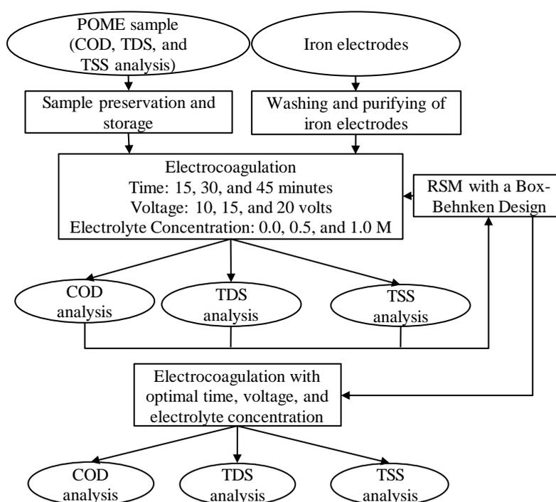
Figure 1 Diagram of the electrocoagulation sequence
