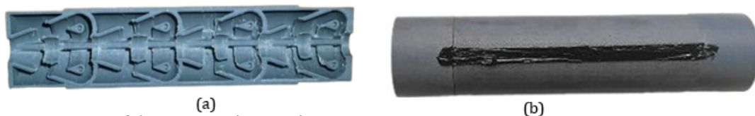
Figure 3 (a) Part of the 3D printed inner silencer result. (b) The two parts are assembled to form the inner silencer
