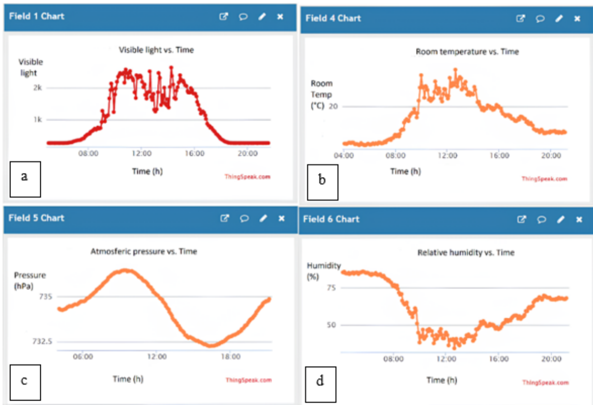
Figure 4 Real-time environmental data obtained from ThingSpeak, including (a) visible light, (b) air temperature, (c) atmospheric pressure, and (d) relative humidity
