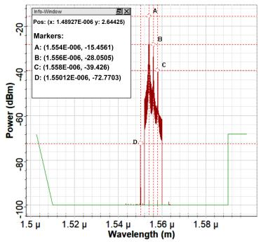
Figure 6 Reflected wavelength outputs from the FBG sensor interrogator under the post-compensation scheme
