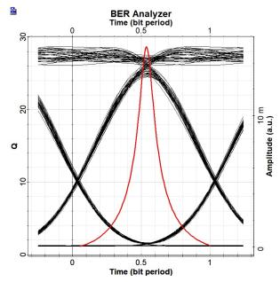
**Figure 4** Eye pattern obtained from the BER analyzer under post compensation configuration with 11 dBm injected optical power
