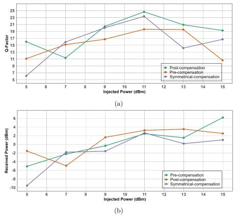
**Figure 3** Comparison of the influence of injected optical power on system performance: (a) injected power vs. Q-factor and (b) injected power vs. received power
