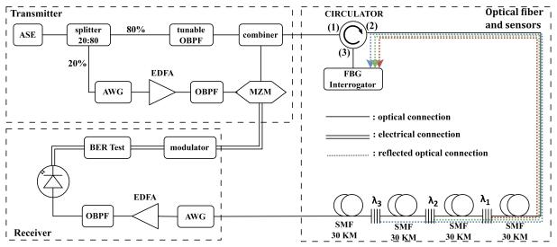
Figure 1 Basic Design of the proposed dual-function optical fiber system integrating high-speed communication and FBG-based sensing
