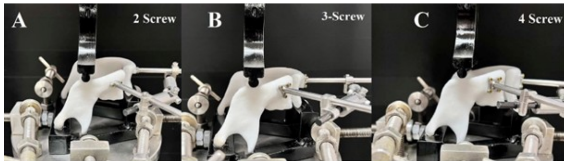
Figure 4 Experimental compression testing of 3D-printed mandible resin models with TEF screw-plate configurations: (A) 2-screw, (B) 3-screw, and (C) 4-screw
