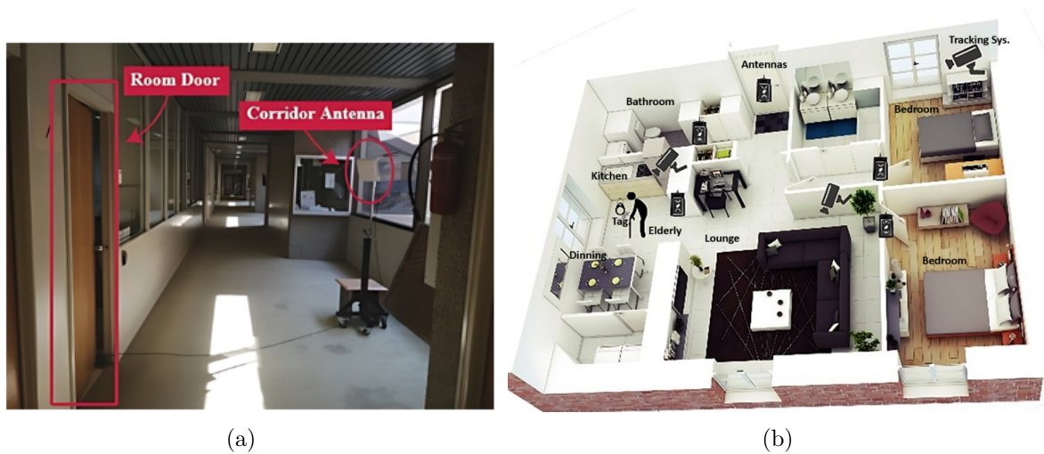
Figure 3 (a) Home control device Antenna setup at the exit, (b) Sample smart home RFID deployment
