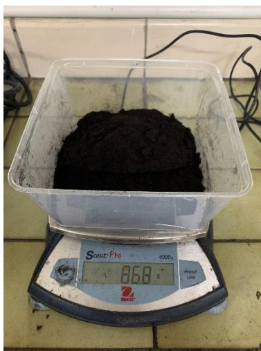
Figure 2 Produced biochar from pyrolysis process.
