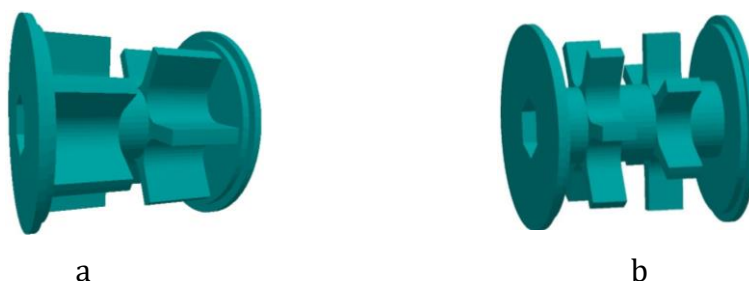
Figure 10 The position of roller gap: a. In the middle; b. In the middle, left, and right sides.
