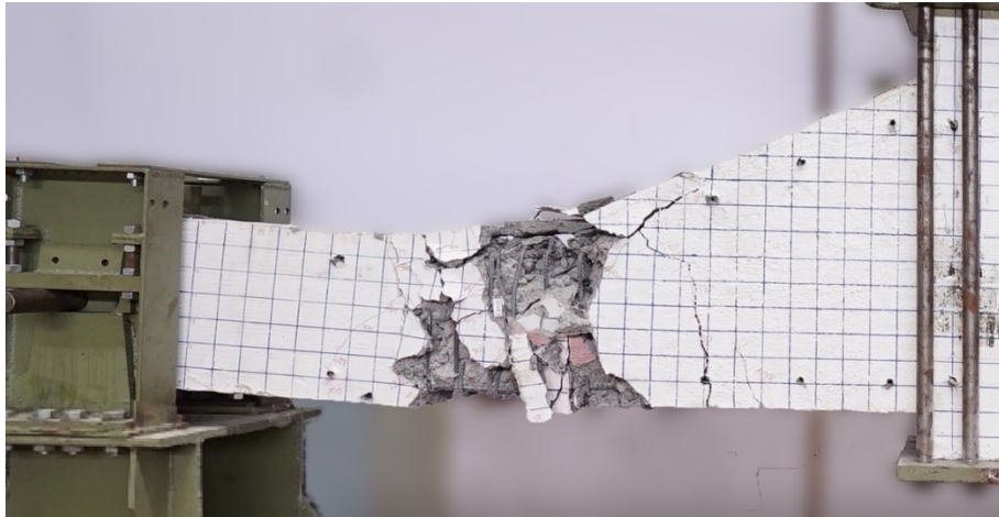
(a) Failure pattern of haunch-strengthened beam-to-column joint.
