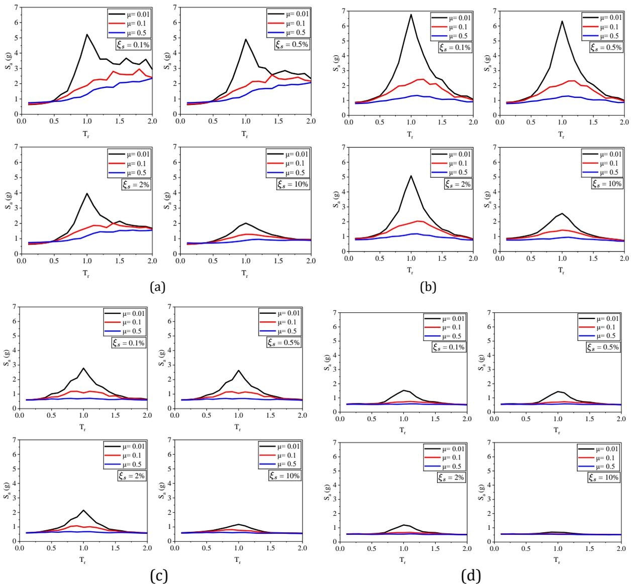
**Figure 5** FRS Vs. tuning ratio under near-field records for (a)  $T_p = 0.1$  sec, (b)  $T_p = 0.5$  sec, (c)  $T_p = 1$  sec, (d)  $T_p = 2$  sec
