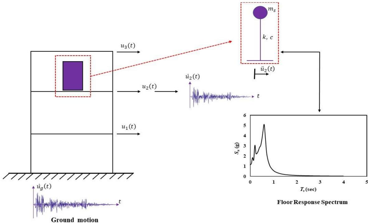
Figure 2 The process of creating floor response spectrum using uncoupled analysis
