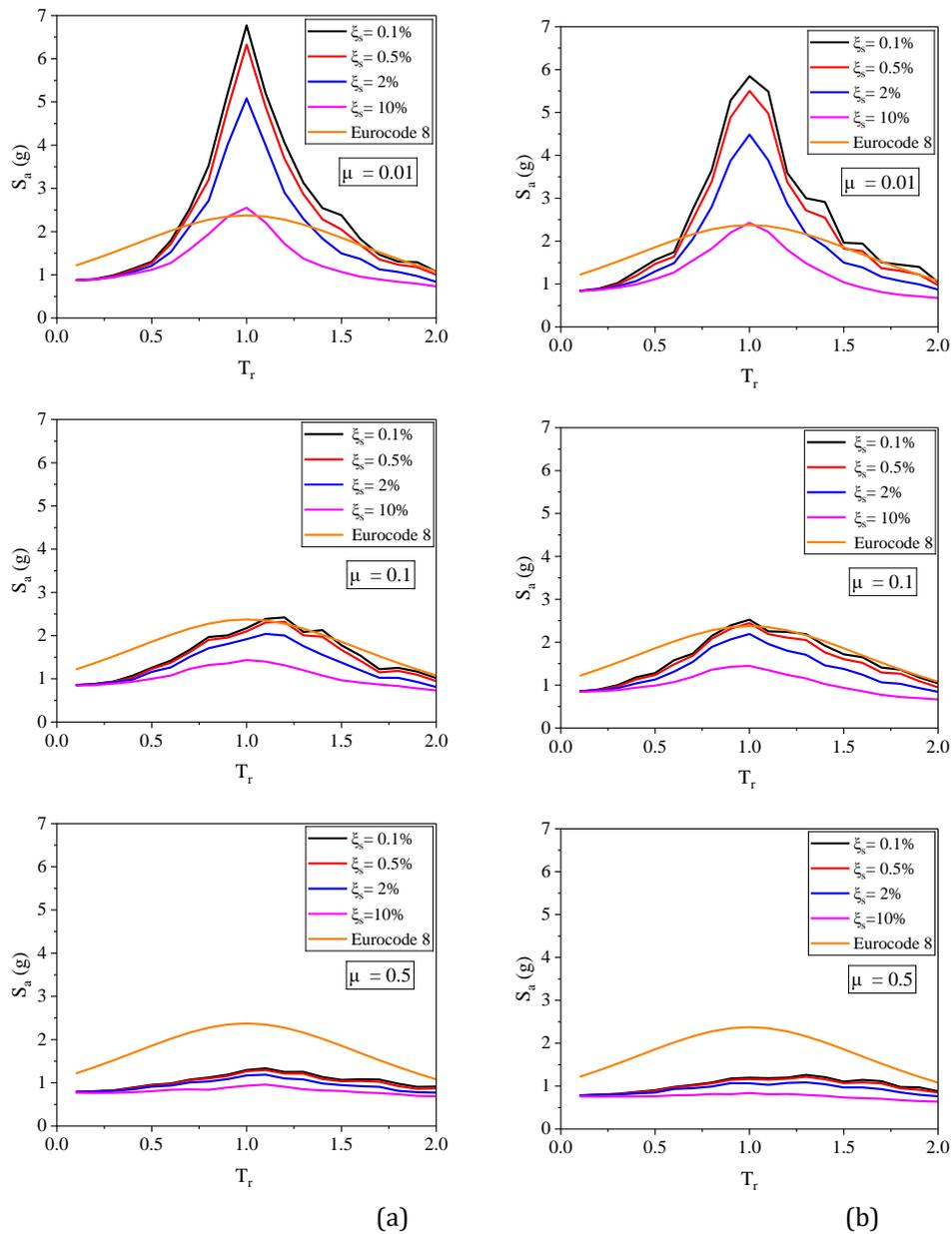
**Figure 7** Comparing the predicted FRS of a PS ( $T_p = 0.5$  sec) with code-based FRS for (a) near-field records and (b) far-field records
