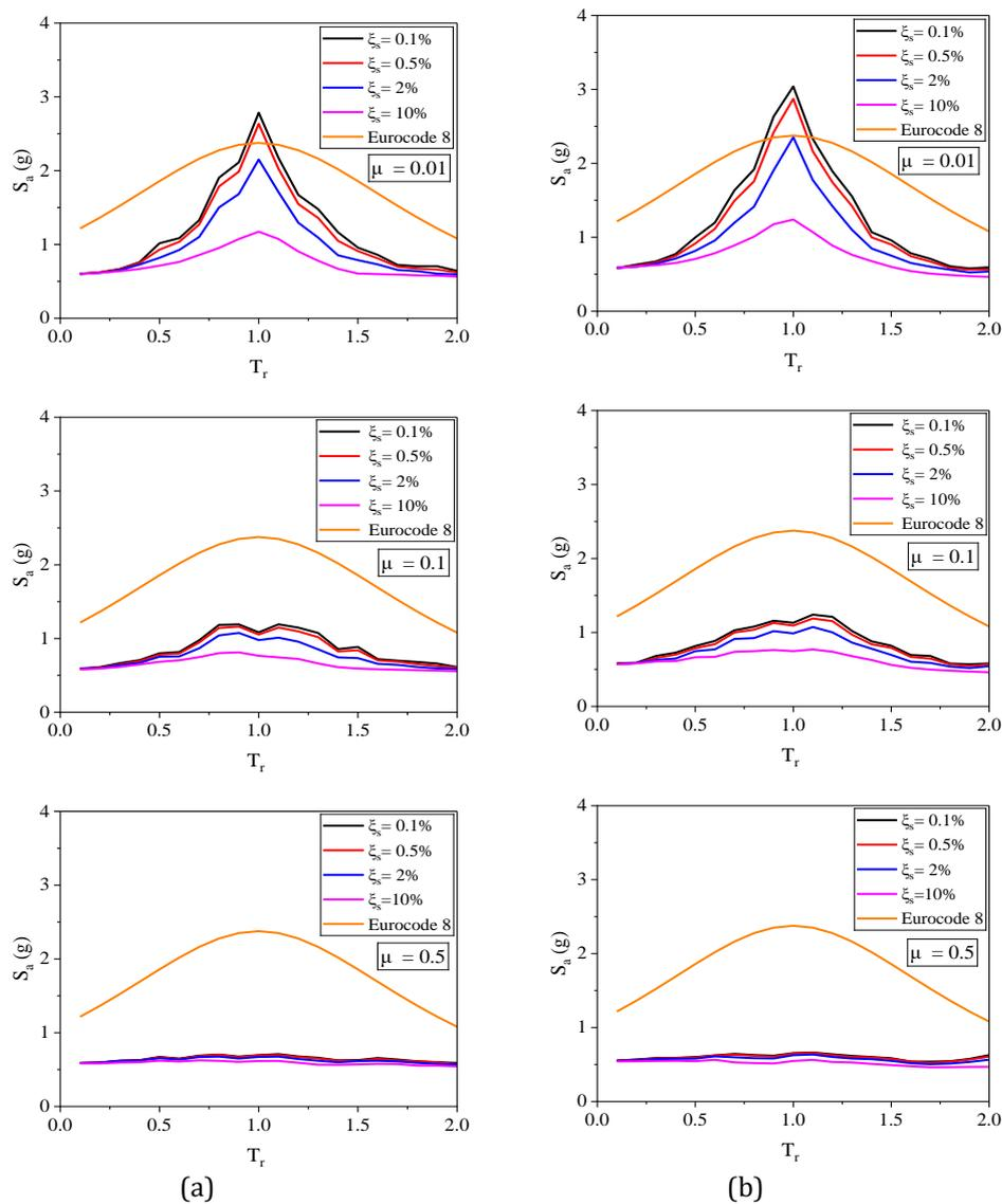
**Figure 8** Comparing the predicted FRS of a PS ( $T_p = 1$  sec) with code-based FRS for (a) near-field records and (b) far-field records
