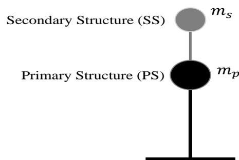
**Figure 1** Secondary structure attached to a Primary structure
