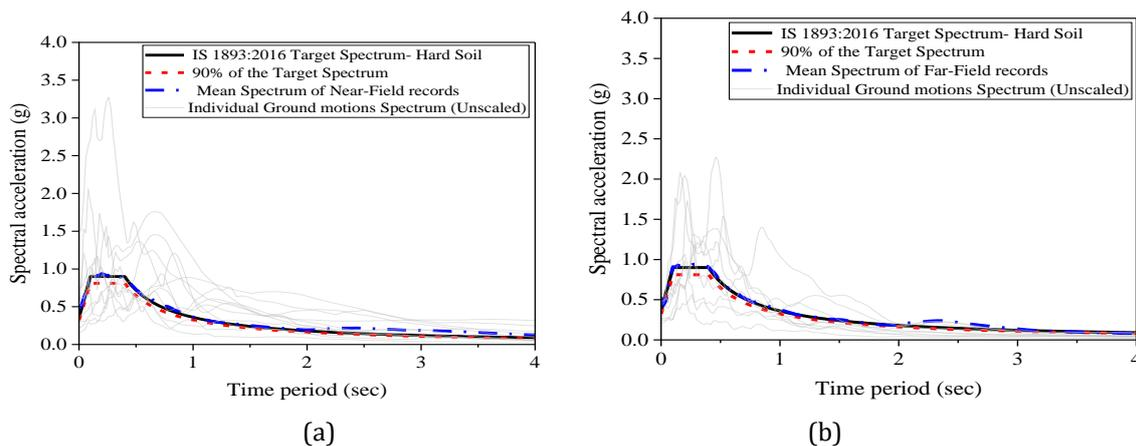
**Figure 3** Scaled ground motions mean spectra and the target spectrum (a) near-field data, (b) far-field data
