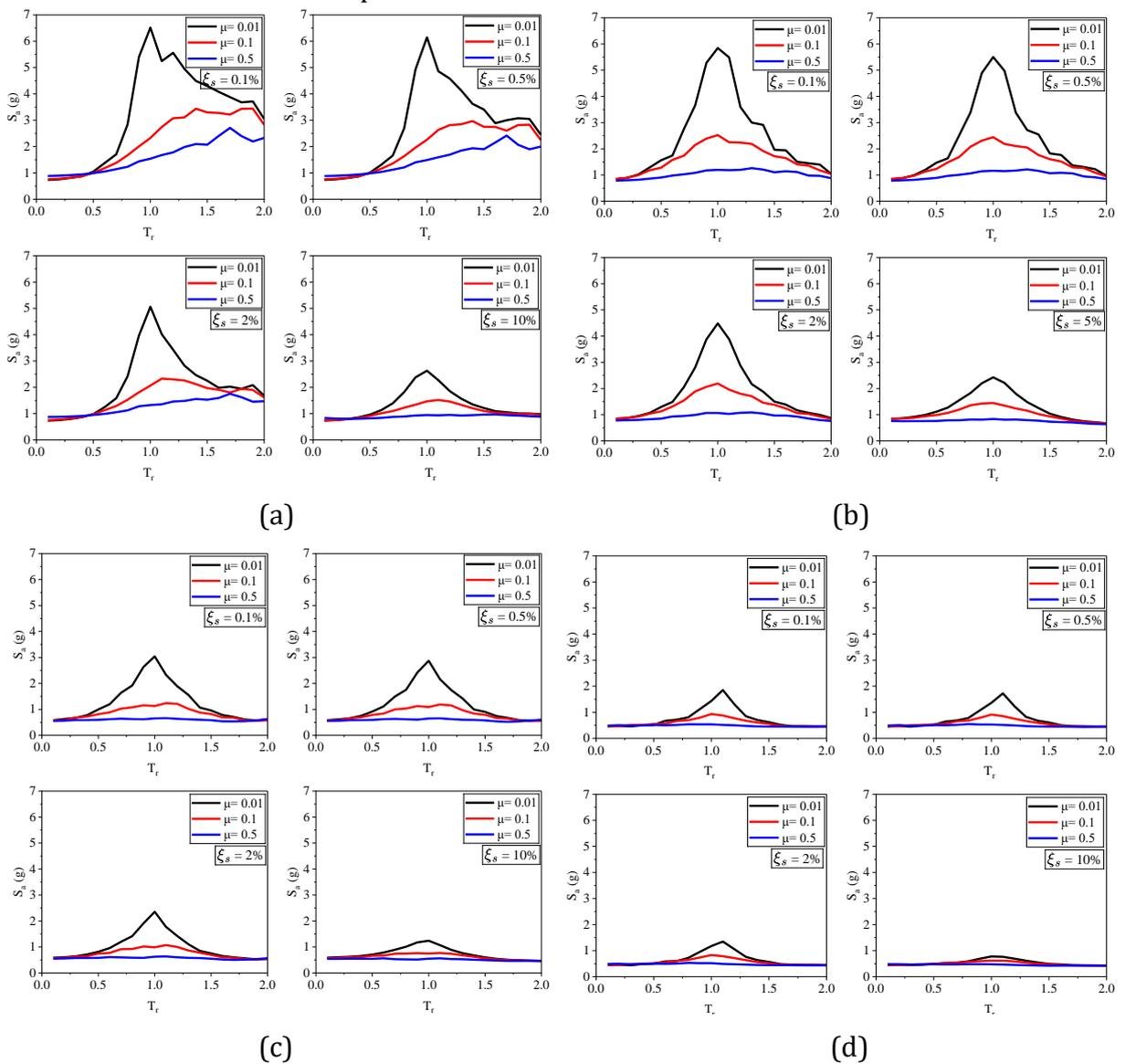
**Figure 6** FRS Vs. tuning ratio under far-field records for (a)  $T_p = 0.1$  sec, (b)  $T_p = 0.5$  sec, (c)  $T_p = 1$  sec, (d)  $T_p = 2$  sec
