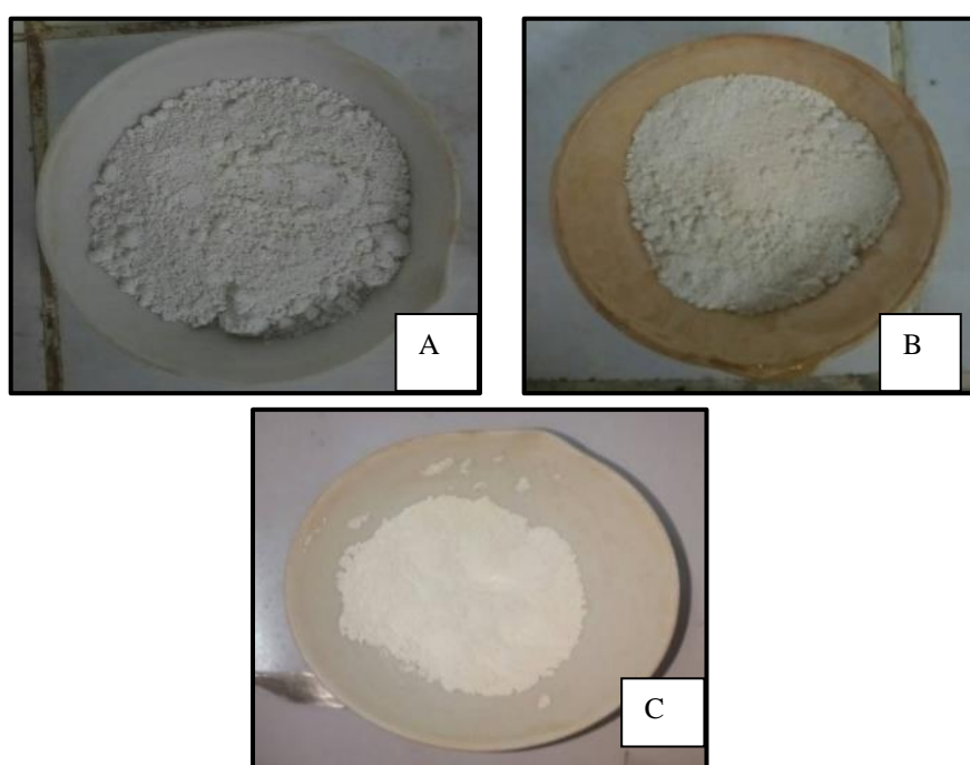
Figure 1 Preparation of (A) natural kaolin 150 mesh, (B) kaolin after oven heating, and (C) kaolin after calcination (metakaolin)
