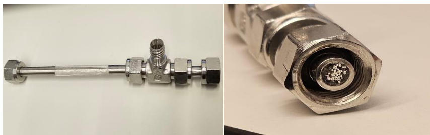
Figure 1 A membrane module for studying the gas transport characteristics of hollow-fiber gas separation membranes
