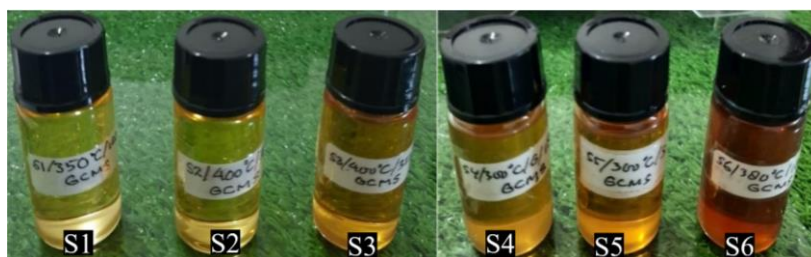
Figure 2 Six samples of PDO of mixed five types of plastic pyrolysis and distillation
