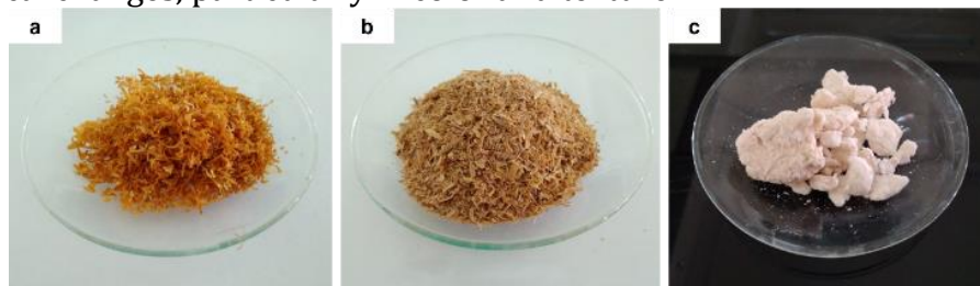
Figure 1 Physical appearance of isolated husk rice fibers for (a) RH, (b) RH_Al, and (c) RH_Al-BI
