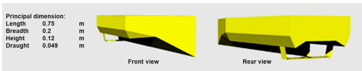
Figure 1 Fast patrol boat design with flat plate hull with duct vane
