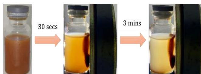
Figure 7 Magnetism test of magnetite mesoporous silica nanoparticle suspension in water (sample E)
