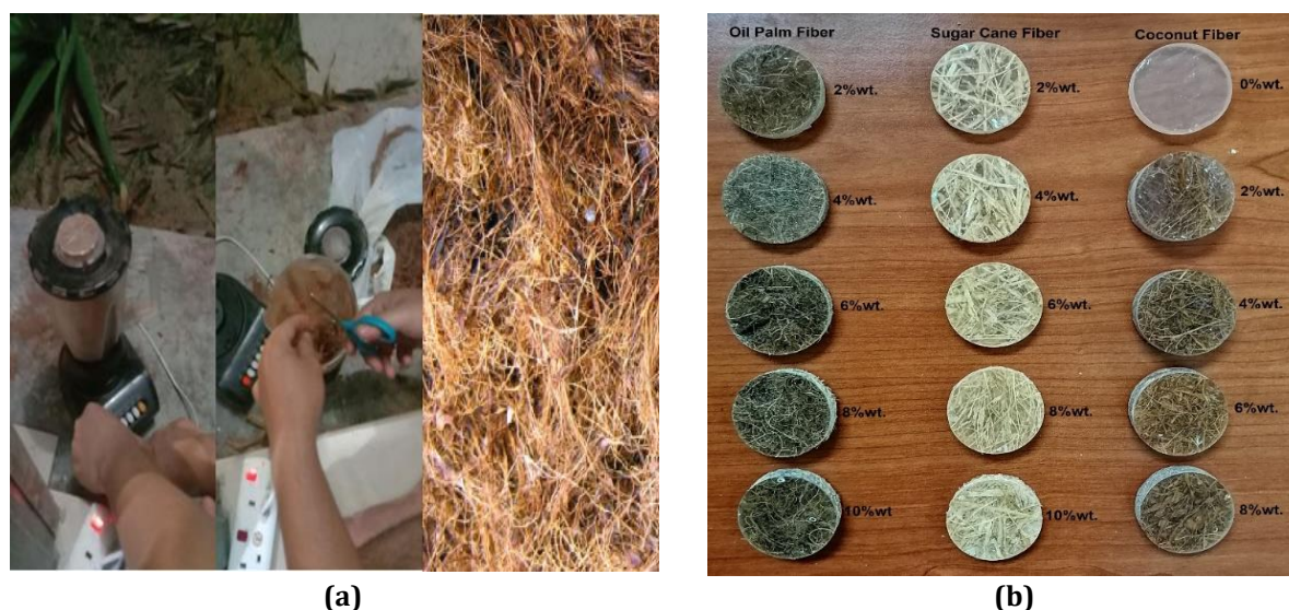
Figure 2 (a) Impurities removal processing, (b) Composite samples were analyzed in the impedance tube
