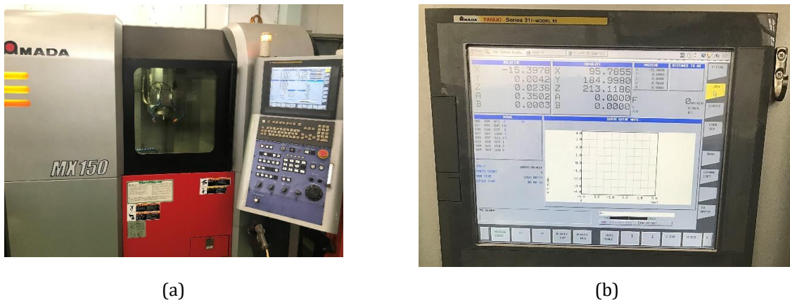
Figure 3 (a) Experimental CNC machine tool; and (b) Integrated FANUC servo guide into the machine for data acquisition
