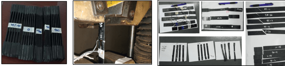
Figure 8 Tensile test material carbon composite produced by the VARI method. (a) Specimens before the test, (b) Tensile test machine, (c) Specimens after the test.
