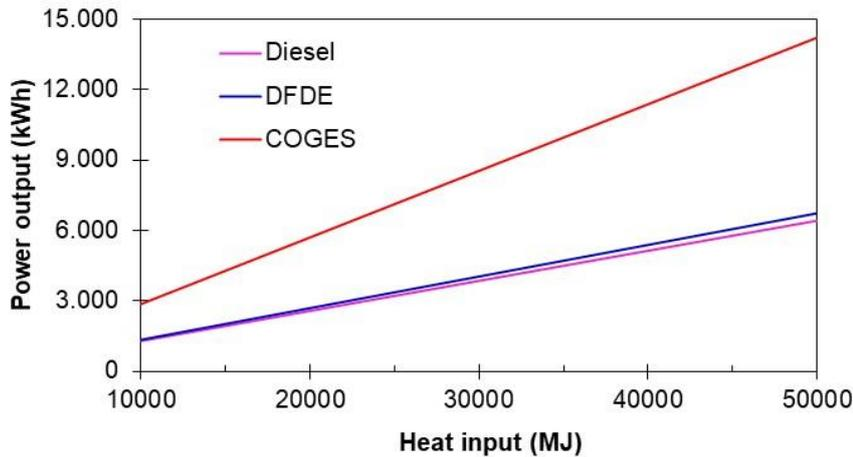
Figure 5 Comparison of the power output from the 3 different propulsion systems
