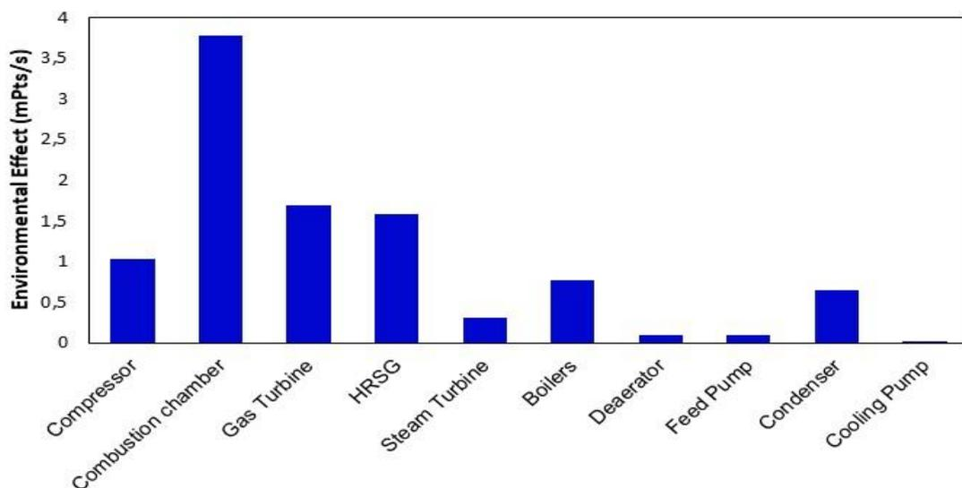
**Figure 7** Environmental impact assessment of COGES propulsion system
