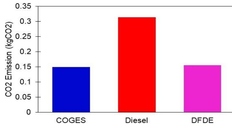
**Figure 6** Comparison Graph of Propulsion System Emissions
