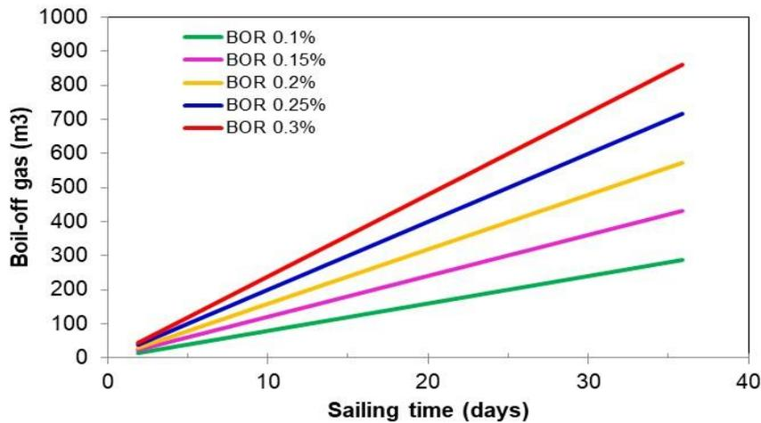
Figure 4 Variation of boil-off of gas results during sailing time
