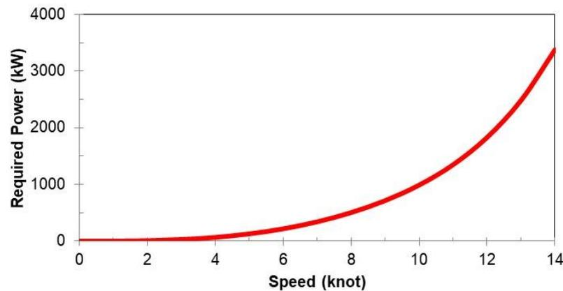
**Figure 1** The required power at the desired speed of the case study
