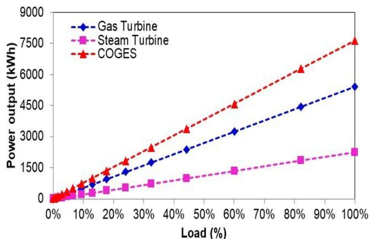
**Figure 3** The power output of the COGES propulsion system
