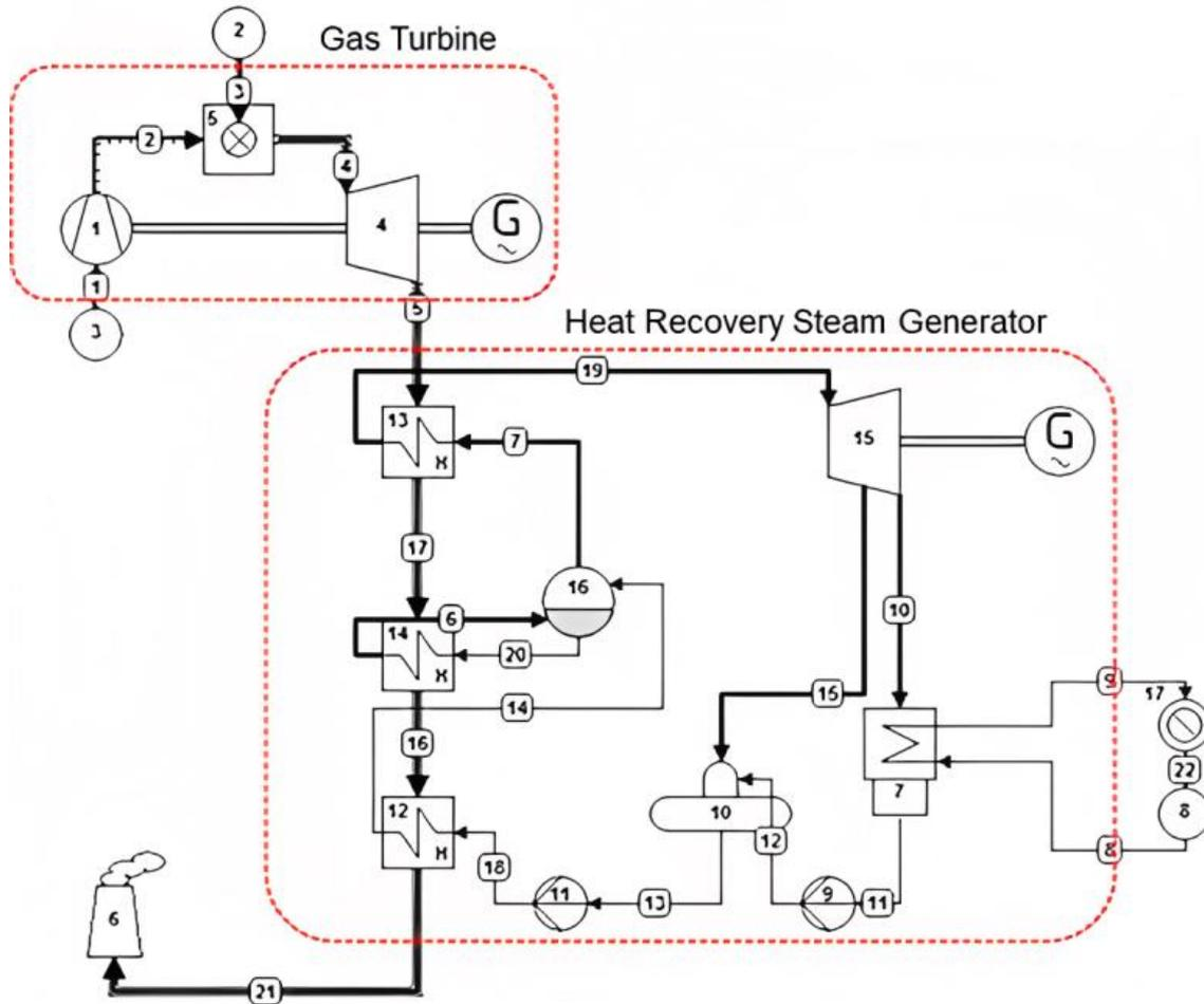
**Figure 2** Proposed design of COGES propulsion system
