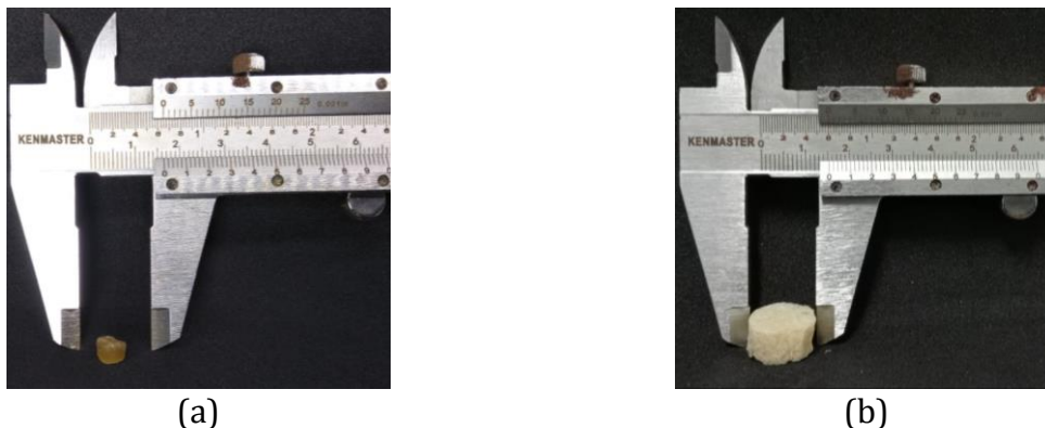
Figure 3 Result of Oven Drying (a) and Freeze Drying (b) of Chi-MA Gels
