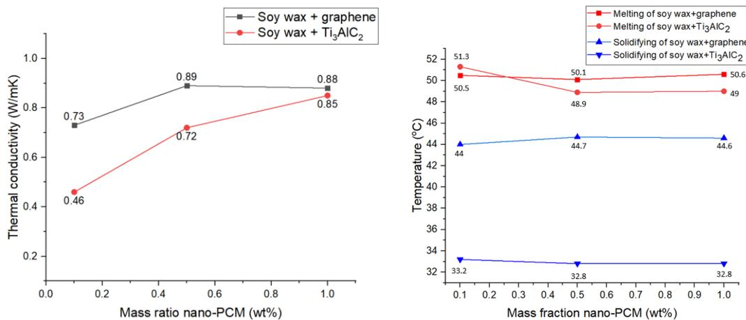
**Figure 5** (a) The enhancement percentage of thermal conductivity of soy wax + graphene and soy wax + Ti<sub>3</sub>AlC<sub>2</sub>, (b) Effect of nanoparticles on melting and solidification temperatures of nano-PCMs
