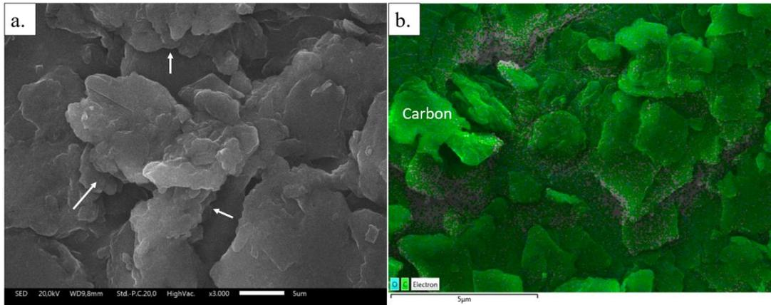
**Figure 3** (a). Morphology of a mixture of soy wax and graphene nanoparticles; (b) mapping distribution elements of graphene
