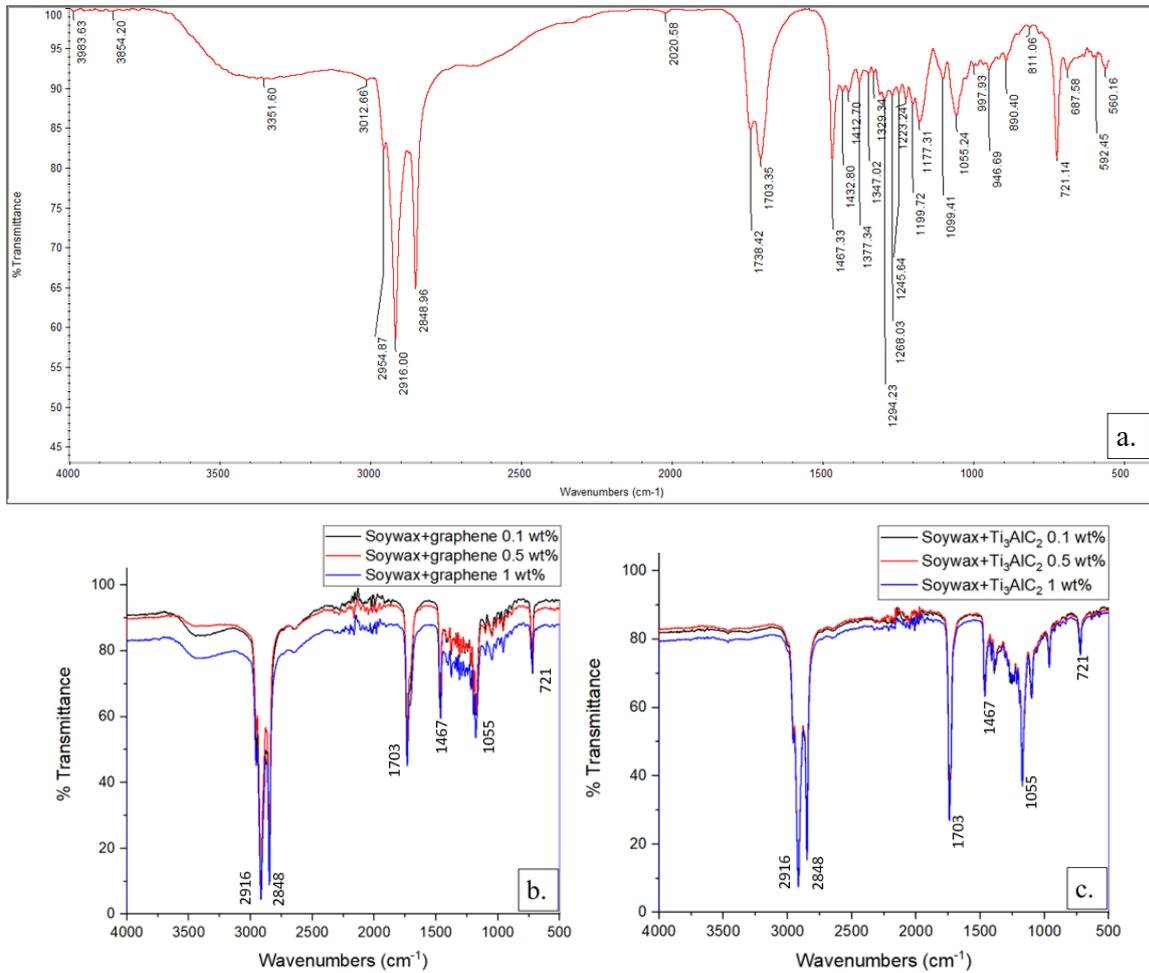
**Figure 2** FTIR spectra of pure soy wax (a), soy wax + graphene (b), soy wax + Ti<sub>3</sub>AlC<sub>2</sub> (c)
