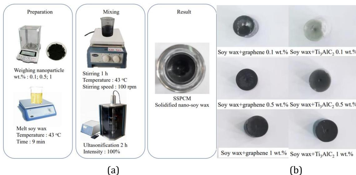
**Figure 1** Nano-PCM synthesis process (a), Synthesis of soy wax+graphene & soy wax+Ti<sub>3</sub>AlC<sub>2</sub> (b)
