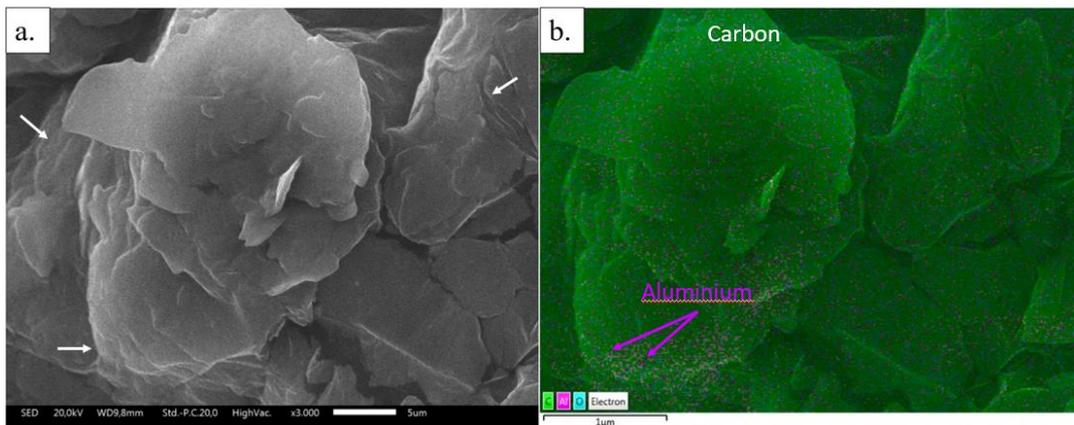
**Figure 4** (a). Morphology of a mixture of soy wax and  $Ti_3AlC_2$  nanoparticles; (b) mapping distribution elements of  $Ti_3AlC_2$
