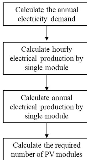
**Figure 2** Flowchart to determine the capacity of PV module for strategy A
