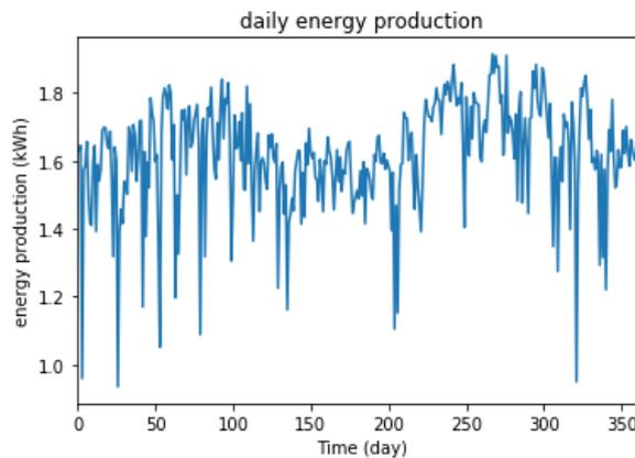
**Figure 5** Simulation result on daily usable energy production from a single PV module for a year
