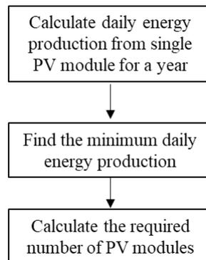
**Figure 3** Flowchart to determine PV module capacity for strategy B
