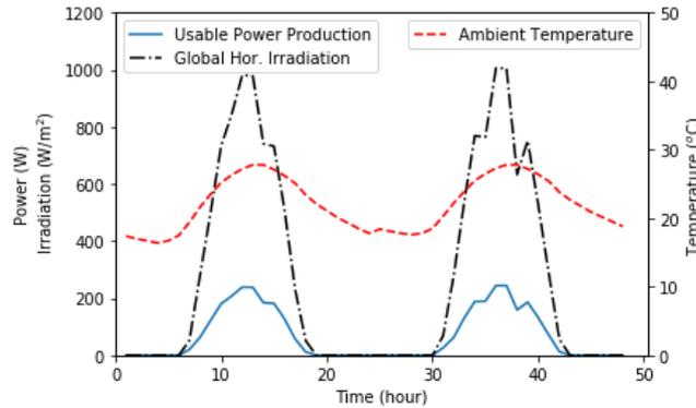
**Figure 4** Simulation result of the usable power production based on the weather conditions
