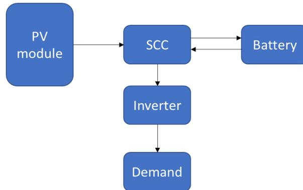
**Figure 1** Configuration of off-grid PV system
