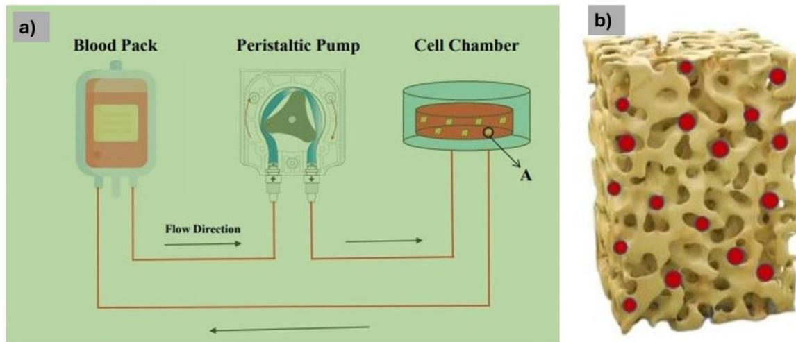
**Figure 1** (a) An illustration of a closed-circuit SHiNTA with a bioreactor inside an incubator. Arrow: Flow direction of complete hepatocyte medium (b) An illustration of cell distribution inside a liver scaffold
