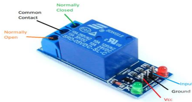
Figure 4 5V DC single channel relay module
