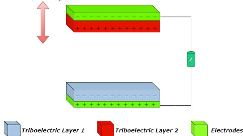
**Figure 1** A schematic illustration of the vertical contact-separation mode
