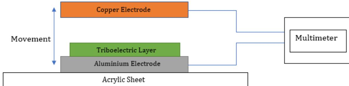
**Figure 6** Schematic diagram demonstrating the experimental setup used for this research
