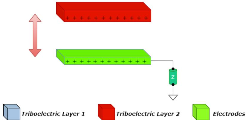
**Figure 3** Schematic illustration of single-electrode mode
