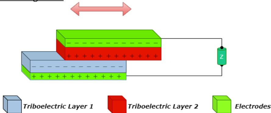
**Figure 2** Schematic illustration of the linear-sliding mode
