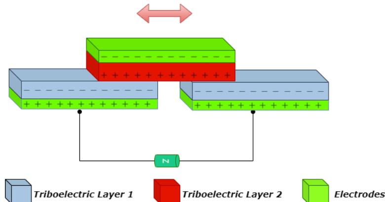
**Figure 4** Schematic illustration of the freestanding triboelectric-layer mode
