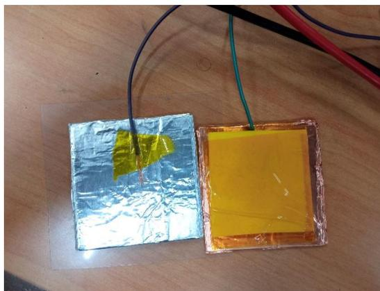
**Figure 7** An example of the experimental set-up. Here it shows the two electrodes made of aluminium, copper, and Kapton being the triboelectric layer
