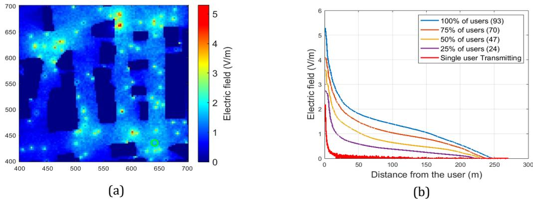
**Figure 5** (a) Spatial distribution of total E-field strength for uplink, (b) Total E-field strength versus distance from the user
