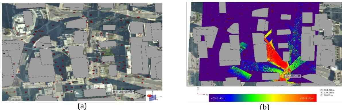
**Figure 2** (a) Location of base-station and random users' locations in a dense urban environment, (b) Received power heatmap for a single beam directed towards a user located near the middle of the map
