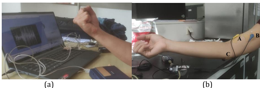
Figure 6 (a) Set-up of EMG signal measurement with FlexComp Infiniti – 10 Channel System device (b) the placement of the EMG measurement probe for the detection electrodes is placed on A and B while the reference electrode is placed on C
