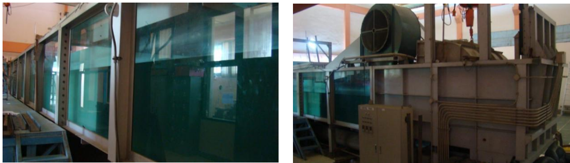
Figure 3 (a) Flume tank; (b) wave generator
