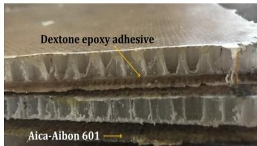
**Figure 3** Bottom-part sandwich composite panels with S<sub>A-A</sub> adhesives and top-part sandwich composite panels with S<sub>D-E</sub> adhesive
