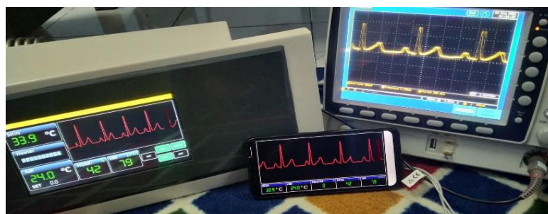
Figure 9 Testing the data transfer based on the IoT system displayed on the LCD display and the android system
