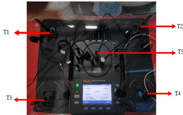
Figure 4 Temperature test using the Incu Analyzer type INCUCU 2 Brand Fluke, with five temperature parameters namely T1, T2, T3, T4 and T5 which are placed as shown in the picture
