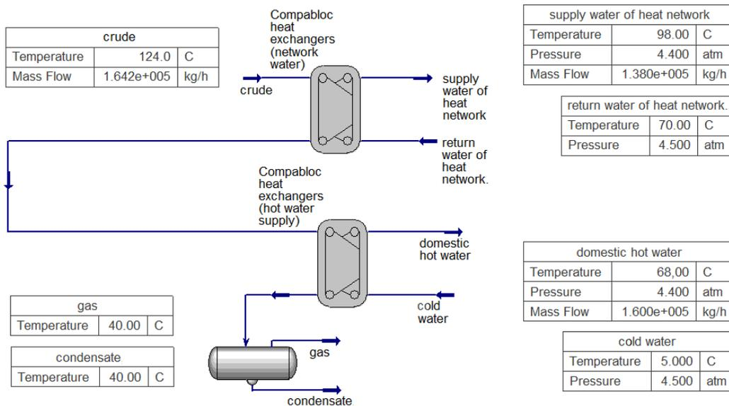
**Figure 4** Water heating model of the hot water supply system and network water using Compabloc heat exchangers
