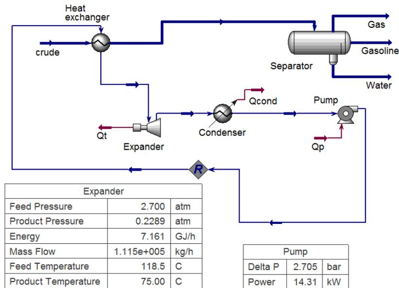
**Figure 6** Organic Rankine cycle installation model without the regenerative heat exchanger
