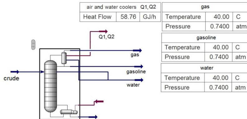
**Figure 1** Column model with the condenser, which simultaneously performs the functions of air coolers, water coolers, and a separator.
