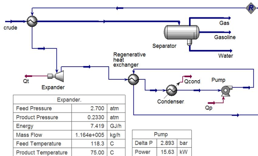
**Figure 5** Organic Rankine cycle installation model with the regenerative heat exchanger
