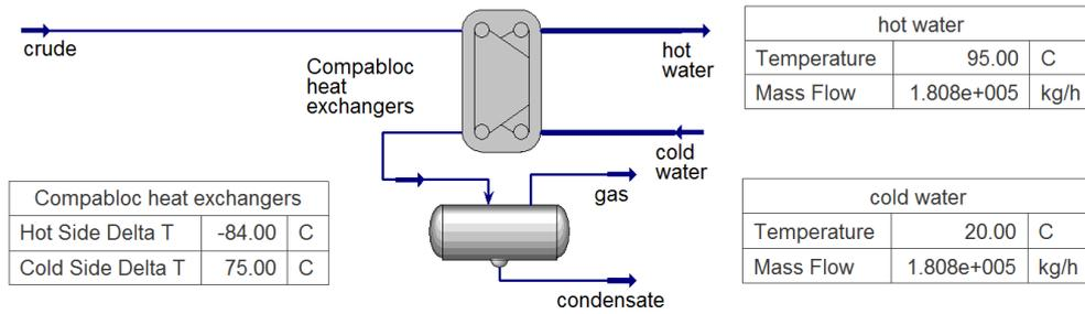
**Figure 3** Model of chemically purified water heating using Compabloc heat exchangers
