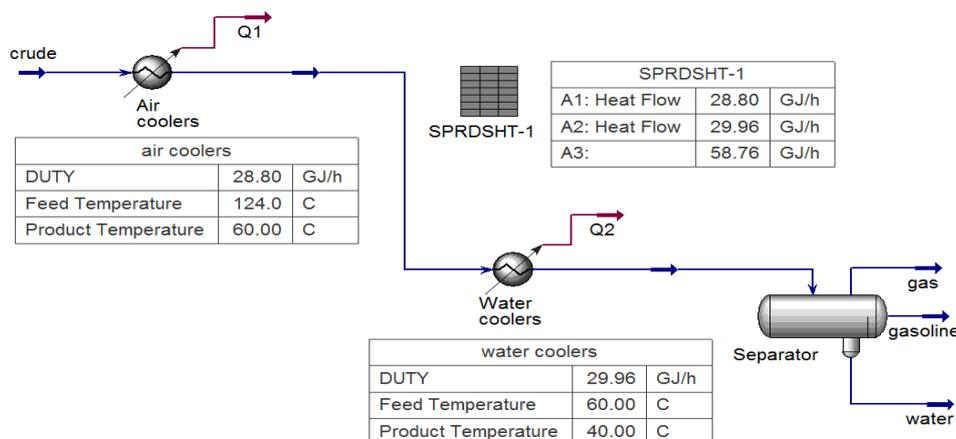
**Figure 2** Scheme of cooling and condensation of the catalytic cracking column overhead vapors with their further separation
