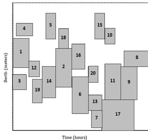
**Figure 4** Illustration for berth plan for 20 vessels in the highly uncertain condition
