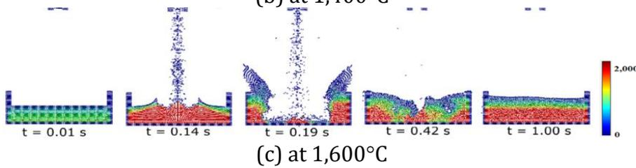
**Figure 10** The pressure profiles of Pb-Al (The unit of pressure is in N/m<sup>2</sup>)
