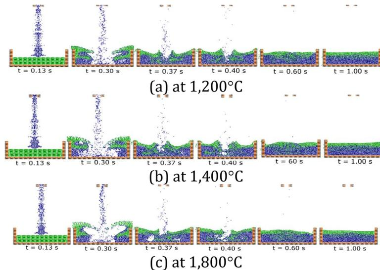
Figure 5 Relocation process of Pb-Al
