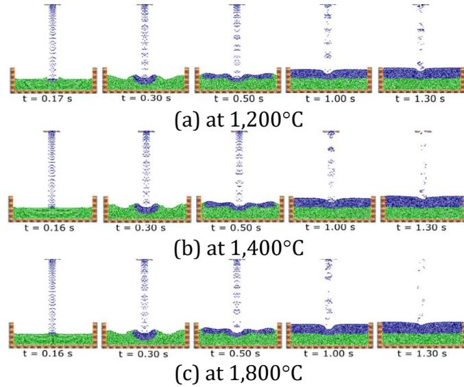
Figure 4 Relocation process of Al-Pb
