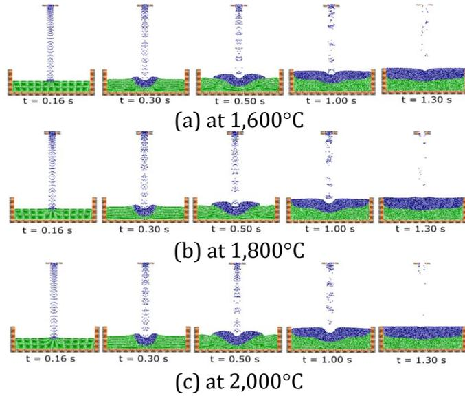
Figure 3 Relocation process of Al-Fe
