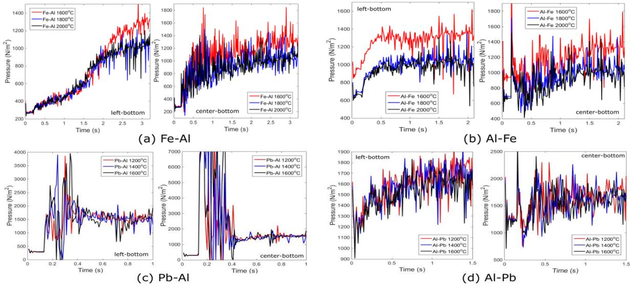
Figure 8 The pressure profiles (in  $N/m^2$ ) inside the container for all configurations
