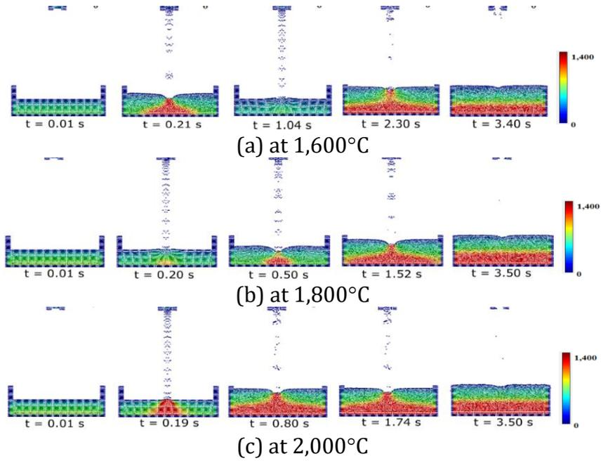
Figure 7 The pressure profiles of Fe-Al (The pressure unit is in  $N/m^2$ )
