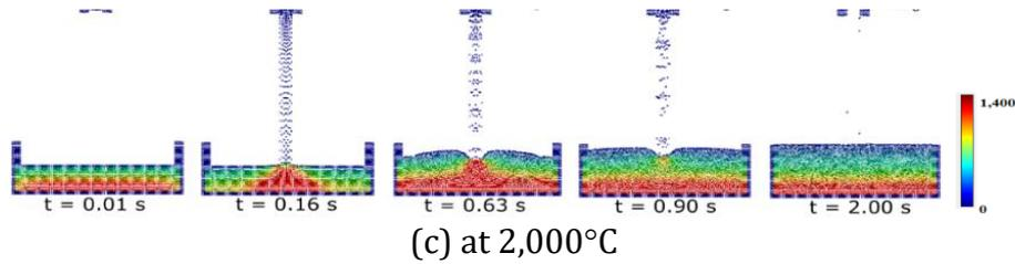
**Figure 9** The pressure profiles of Al-Fe (The unit of pressure is in N/m<sup>2</sup>)
