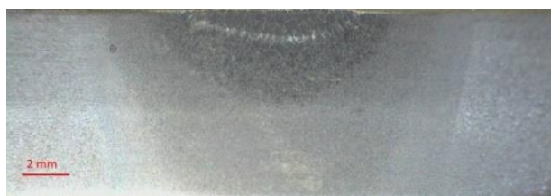
Figure 7 Optical macrograph cross-section of the weld bead for welding current intensity I=100 A (section at 60 mm from the edge of the plate)
