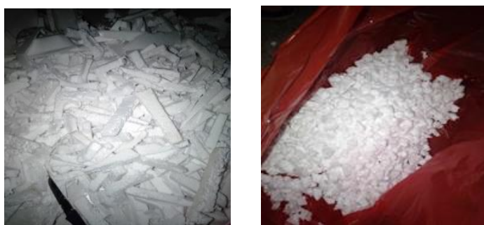
Figure 1 Styrofoam plastic waste as pyrolysis feedstock
