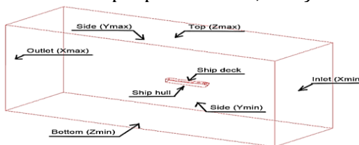
Figure 2 A sketch of the boundary condition
