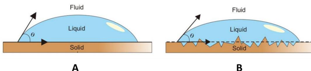
**Figure 8** (A) Young contact angle on an ideal surface and (B) the apparent contact angle on a rough surface
