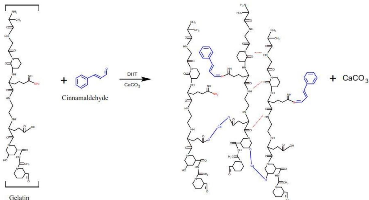
**Figure 4** Synthesis of cinnamaldehyde and CaCO<sub>3</sub> hydrogel, continued by physical crosslinking through de-hydrothermal treatment
