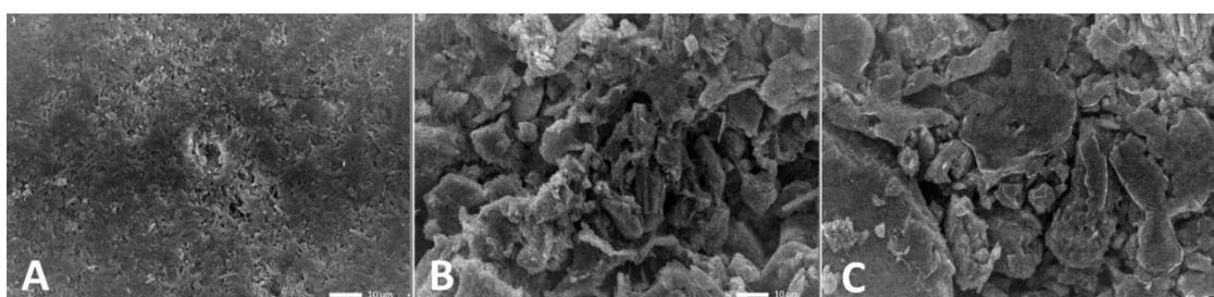
**Figure 7** Scanning electron microscopy of the plaster of Paris composites containing different ratios of CaCO<sub>3</sub> hydrogel. (A) POP-100, (B) POP/HCin-075, and (C) POP/HCin-050 at 1000X magnification
