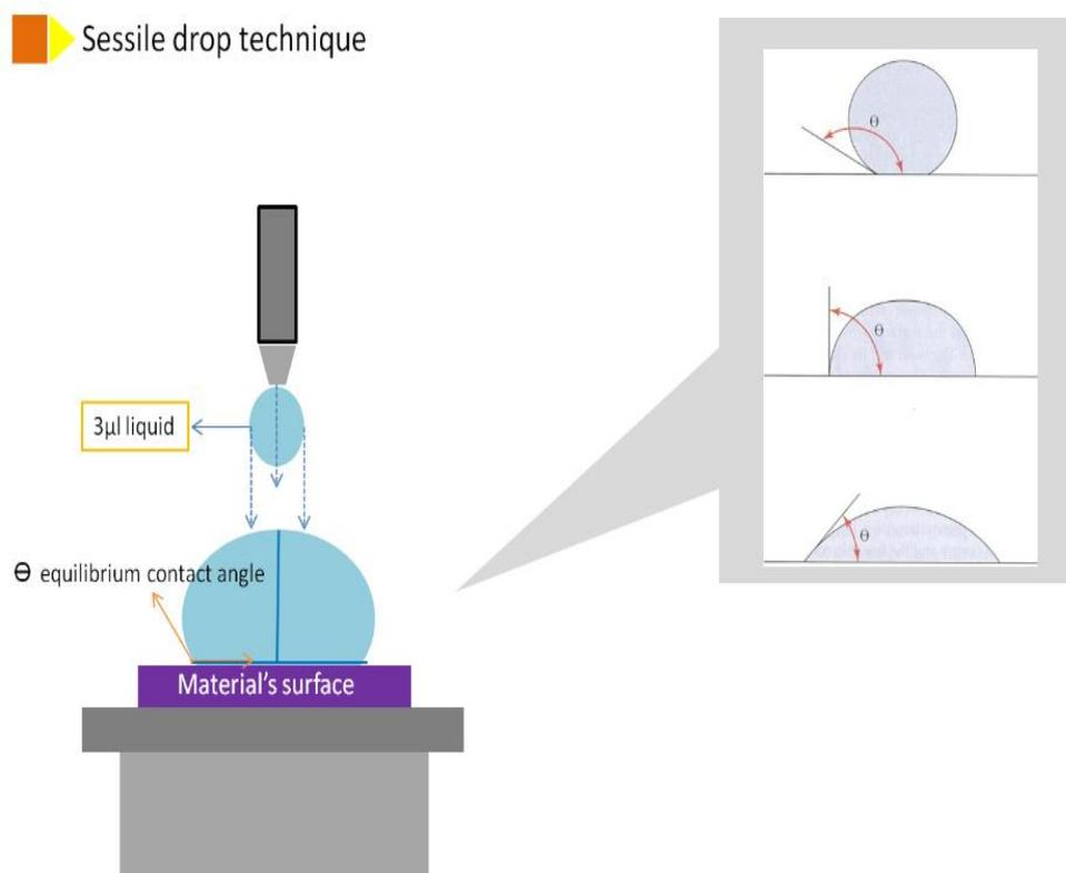
**Figure 2** Schematic of the contact angle measurement process (after Peng and Li, 2014)
