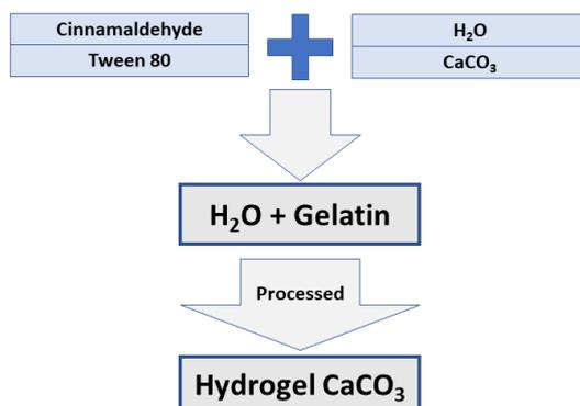
**Figure 1** Procedure for incorporating cinnamaldehyde in a CaCO<sub>3</sub> hydrogel preparation
