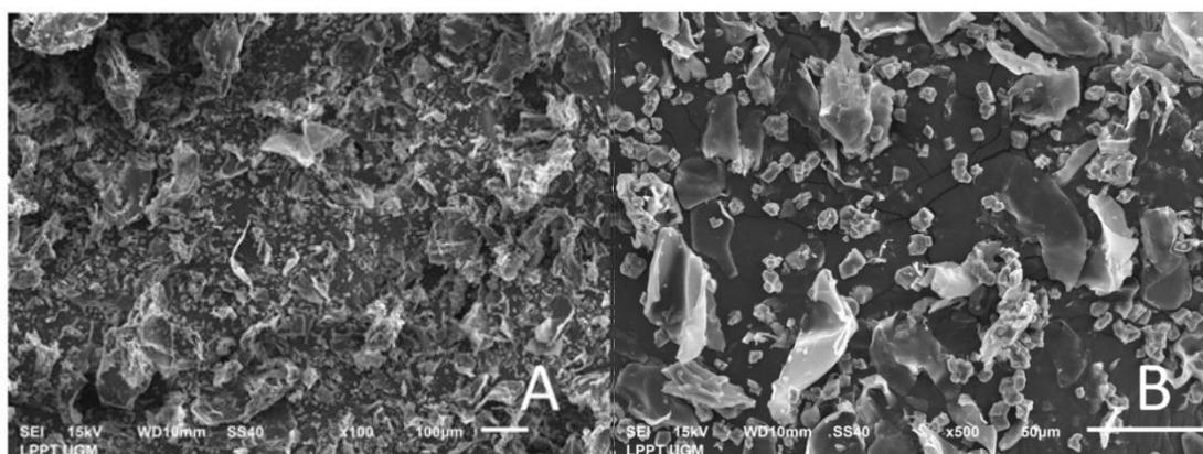
**Figure 6** Scanning electron microscopy of the cinnamaldehyde-loaded CaCO<sub>3</sub> hydrogel at (A) 100× (B) and 500× magnification
