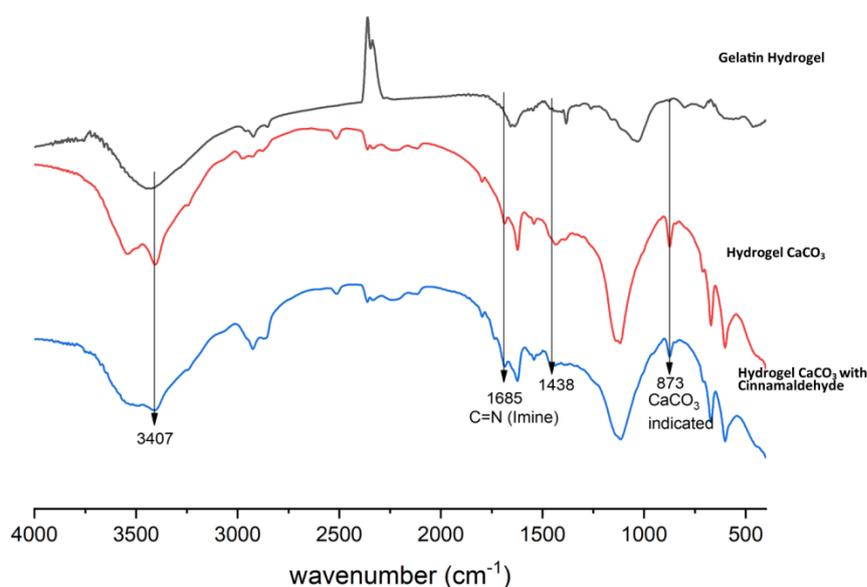
**Figure 5** Fourier transform infrared spectroscopy spectra confirmation of the gelatin hydrogel, CaCO<sub>3</sub> hydrogel, and CaCO<sub>3</sub> hydrogel crosslinked with cinnamaldehyde
