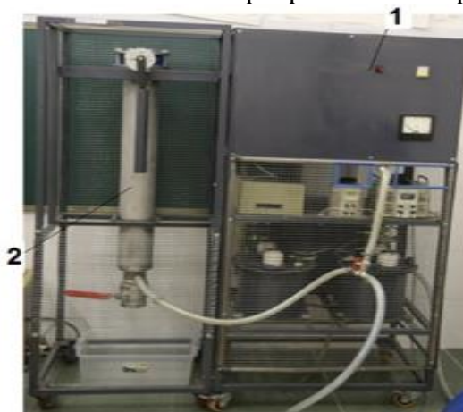
Figure 1 Ion-ozone cavitation installation: (1) ion-ozone generator; (2) cavitation capacity
