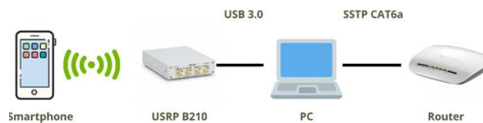
Figure 2 Physical Design of the System
