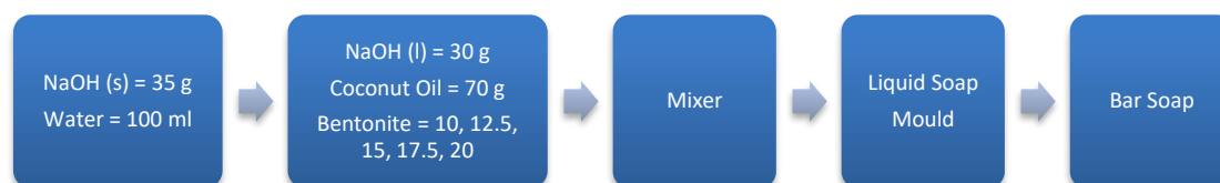
Figure 1 Flow diagram of the process of making bentonite bar soap
