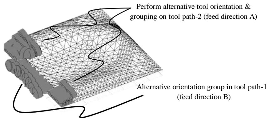
**Figure 20** Results of the peripheral simulation algorithm’s implementation on model-2 surface
