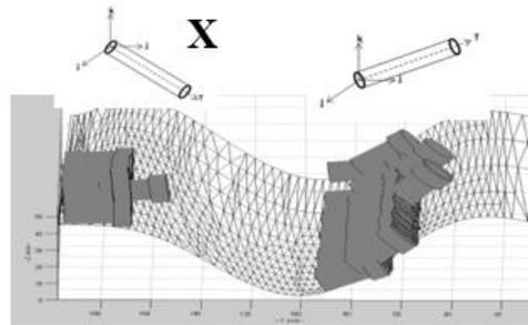
**Figure 10** The orientation tool vector used is based on  $(T_{(i,j,k)})$  as a tool orientation on the surface
