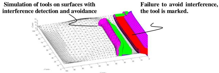
**Figure 17** Orientation after interference detection and avoidance
