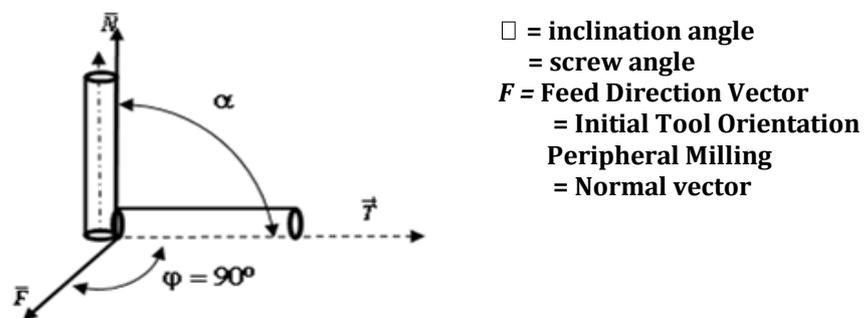
**Figure 5** Determining the tool orientation for the Peripheral milling (Syaefudin et al., 2017)
