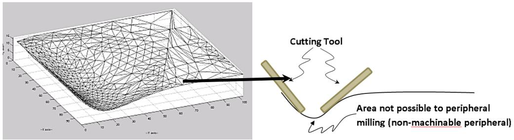
**Figure 13** The area that cannot be peripherally milled (non-machinable)
