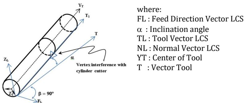
**Figure 7** The vertex inside the tool and the tool inclination system orientation (Kiswanto et al., 2006)
