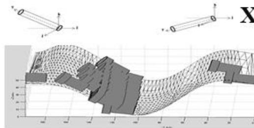
**Figure 11** The reverse tool orientation vector used is based on  $(T_{(i,j,k)})$  as a tool orientation on the surface
