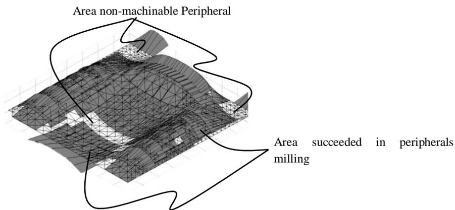
**Figure 21** Marking the peripheral milling area in model-2; the white area is a non-machinable peripheral area
