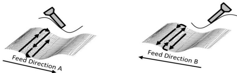
**Figure 12** Grouping the feed direction based on the tool orientation
