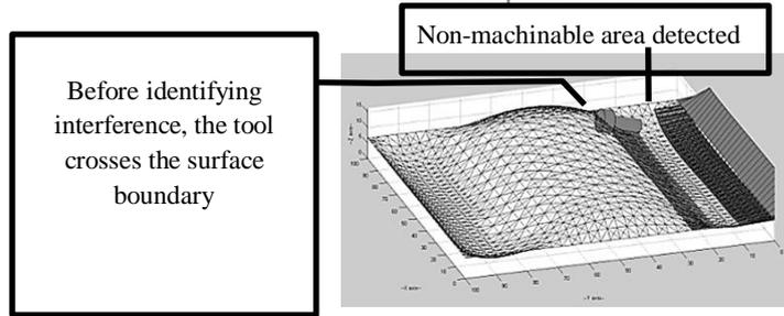
**Figure 16** Milling the whole surface with identification and avoiding collision on model-3 as sample
