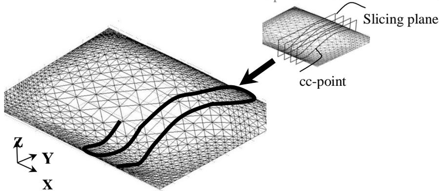
**Figure 6** Creating a tool path on the surface (Kiswanto et al., 2006)
