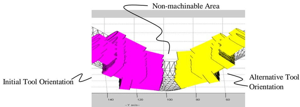
**Figure 19** 3D simulation of the tool orientation for the peripheral milling process
