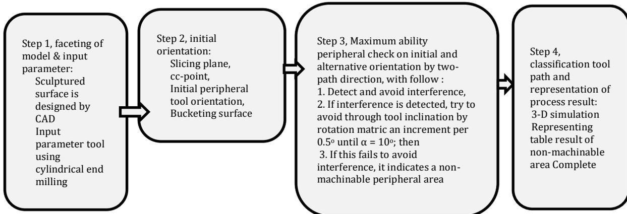
**Figure 2** The method of developing peripheral milling
