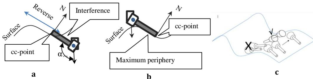
**Figure 9** (a) Orient the initial tool with a large inclination angle; (b) Avoid interference with reverse orientation; (c) Illustration of maximum peripheral tool orientation in 3 dimensions
