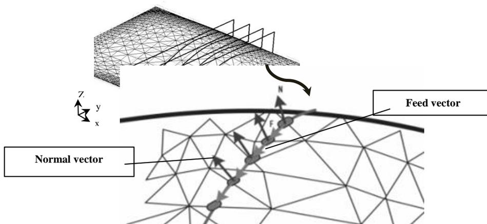
**Figure 3** Determining the normal vector and the feed direction vector (Kiswanto et al., 2006)
