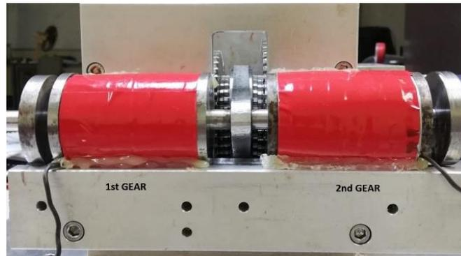
Figure 4 An electromagnetic actuator with 163 coil turns
