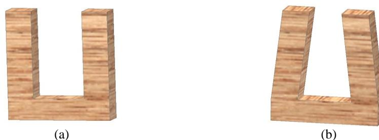
Figure 15 Prong test showing: (a) acceptable piece of board; and (b) unacceptable piece of board with excessive stress build-up
