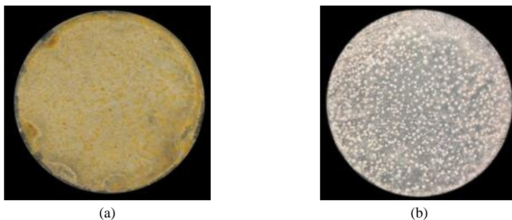
Figure 9 Photographs of low carbon steel surface exposed to corrosion: (a) 0.1 M HCl; and (b) with 0.0004 mol/L of BPTU at 28°C
