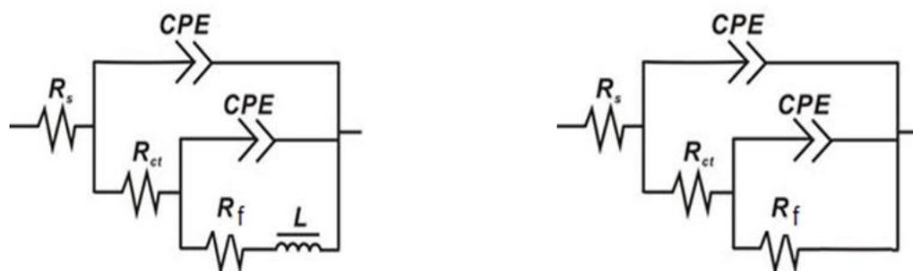
Figure 4 Equivalent circuit used to model the impedance spectra measured on the Mg-5Zn alloys: (a) in  $(\text{NH}_4)_3\text{PO}_4$ ,  $(\text{NH}_4)_3\text{PO}_4 + \text{Succinic Acid}$ , and  $(\text{NH}_4)_3\text{PO}_4 + \text{Malonic Acid}$ ; (b) in NaF, NaF + Succinic Acid and NaF + Malonic Acid
