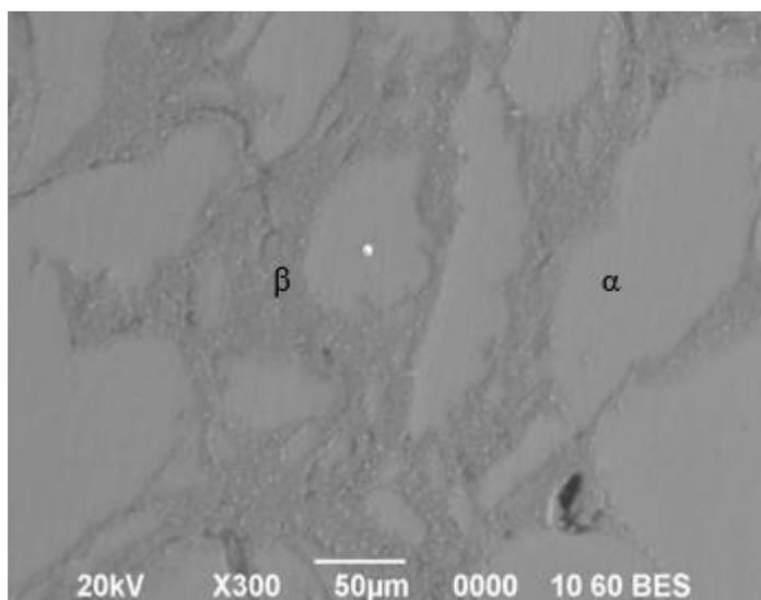
Figure 1 Image of scanning electron microscopy by the back scattering mode of Mg-5Zn shows the  $\beta$  phase in the  $\alpha$  matrix
