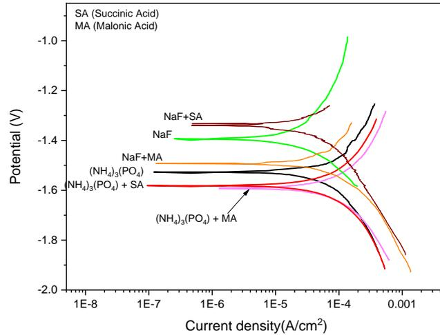
Figure 5 Potentiodynamic polarization curve for Mg-5Zn in 1%  $(\text{NH}_4)_3\text{PO}_4$ , 1% NaF, a binary mixture of 1%  $(\text{NH}_4)_3\text{PO}_4$  with 1% succinic acid and with 1% malonic acid, and a binary mixture of 1% NaF with 1% succinic acid and with 1% malonic acid.
