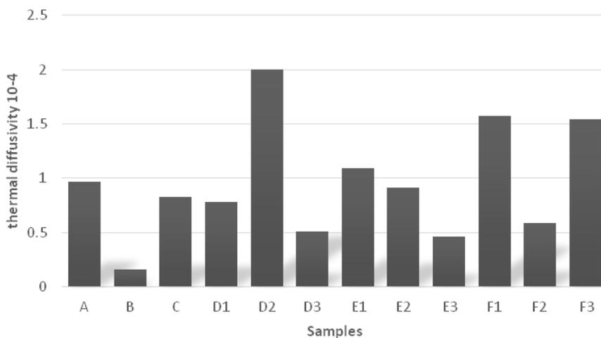
Figure 13 Thermal diffusivity of the developed biomass materials concentration at a constant temperature
