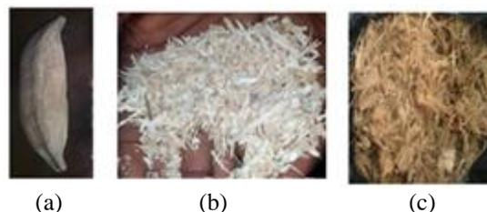
Figure 1 Materials used before processing: (a) Kapok pod; (b) Sugarcane bagasse; and (c) Coconut fibre (coir)
