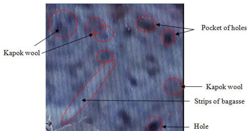
Figure 14 Micrograph of bagasse-Kapok interwoven structure showing pocket of holes ( $\times 150$ )
