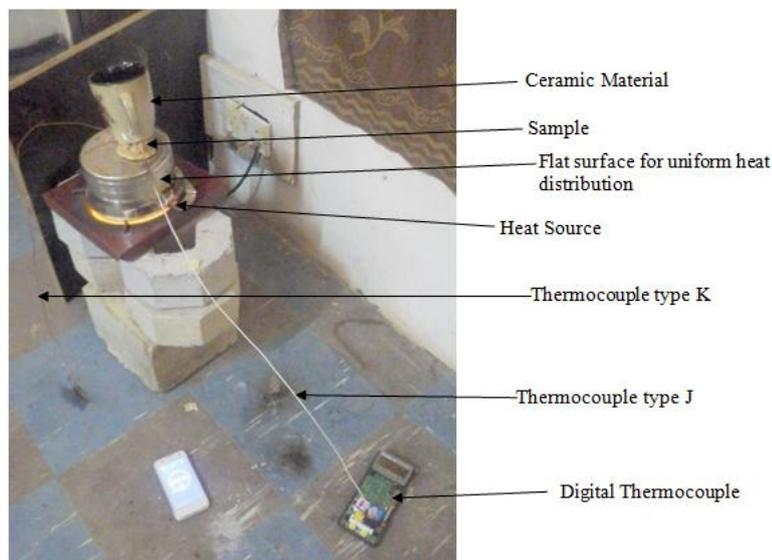
Figure 9 Experimental setup
