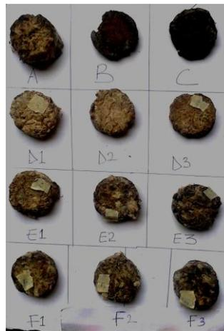
Figure 5 Moulded biomass composites
