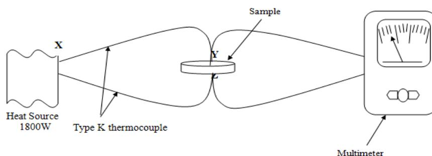
Figure 6 Schematic diagram of thermal conductivity experiment
