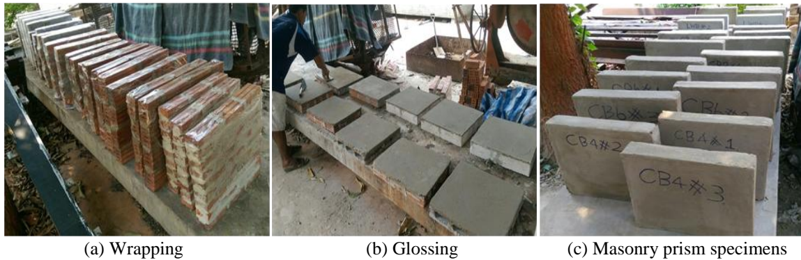
Figure 3 Preparing masonry prism specimens
