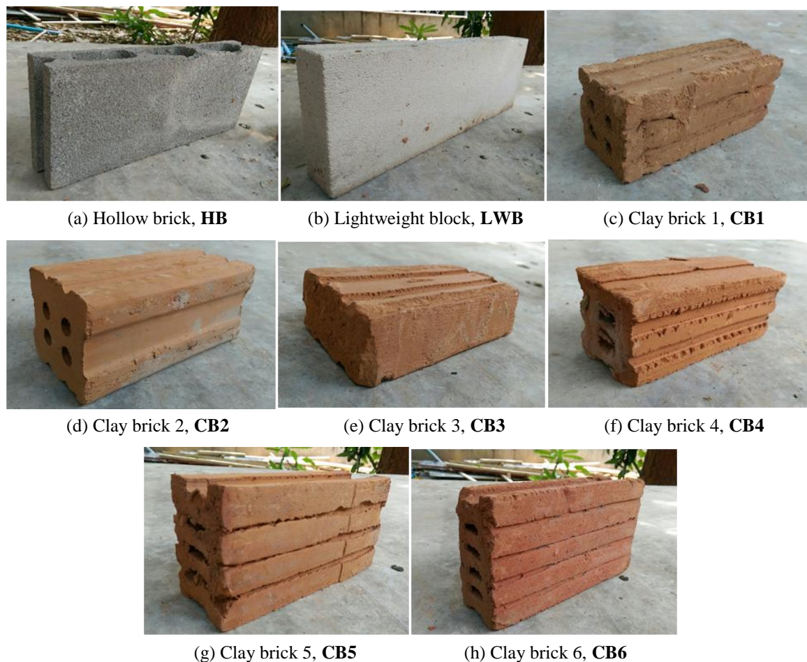
Figure 2 Eight types of brick specimens
