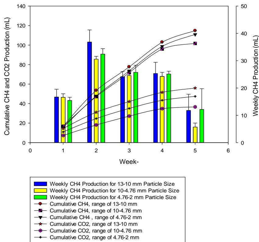
Figure 2 Comparison chart for the cumulative volume of CH<sub>4</sub> and CO<sub>2</sub> with weekly CH<sub>4</sub> production
