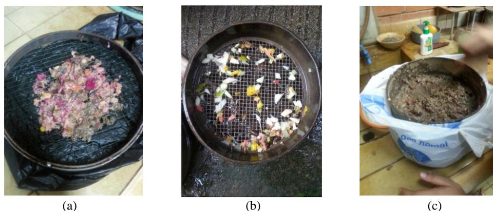
Figure 1 Resulting substrate after chopping and sieving: (a) 10-13 mm; (b) 4.76-10 mm; and (c) 2-4.76 mm
